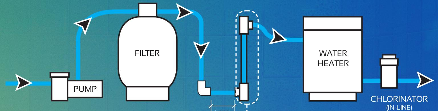
\* Allow a minimum of 12 linear inches of pipe before the UV Light water inlet.
